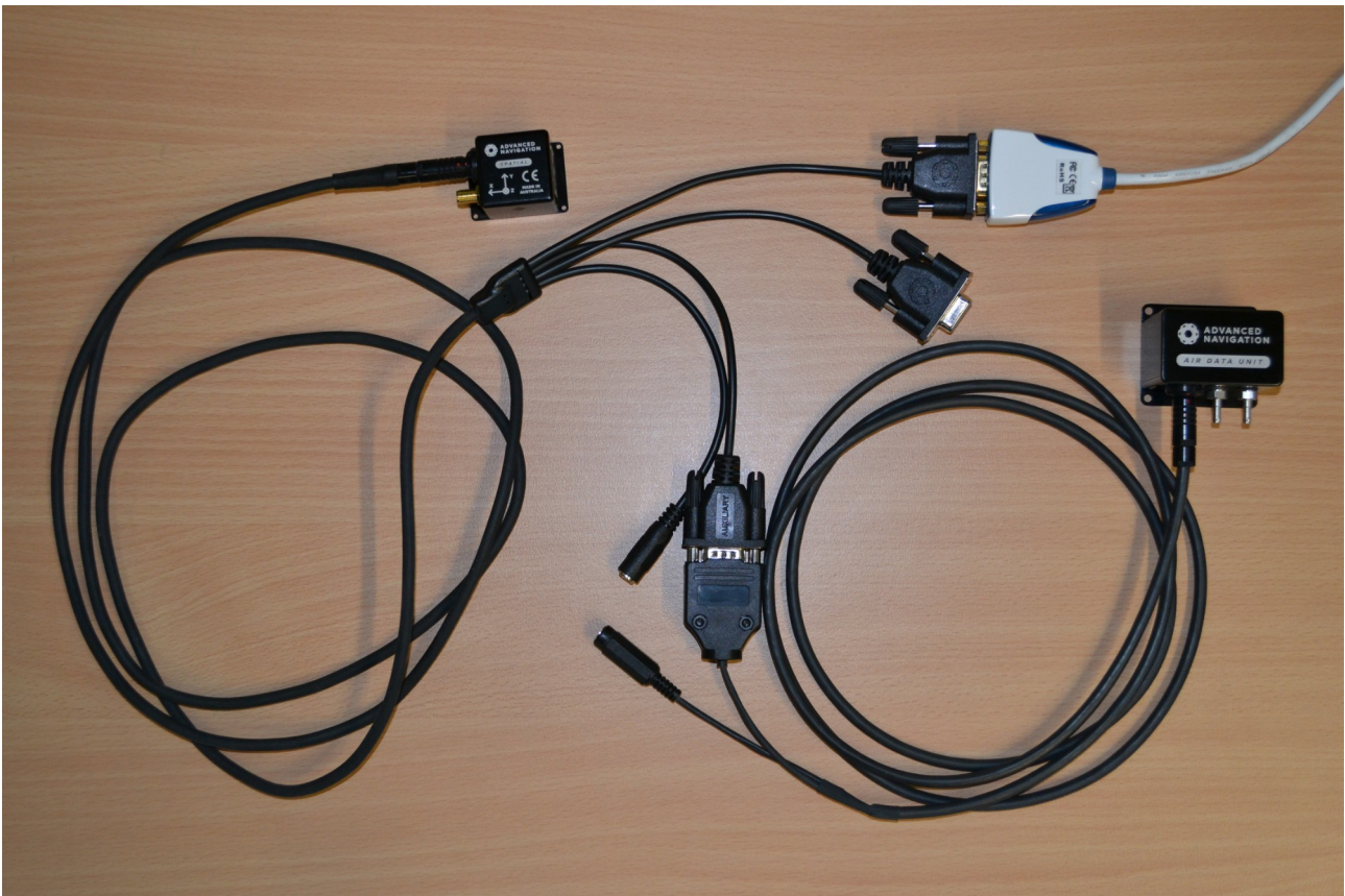
Illustration 8: Air Data Unit connected to Spatial
